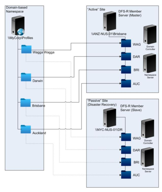
If the DR plan is activated, the DR site's NUS is up-to-date with the changes replicated from the master NUS. However, the namespace server still reflects the wrong view of the namespace, so its configuration must be updated. For each folder, the folder target on the master site must be disabled and the folder target on the DR site enabled.
